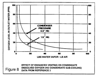
ppb of dissolved oxygen; a water vapor/air ratio of approximately 65 reduces the oxygen content of the condensate to an acceptable level of 7 ppb.
